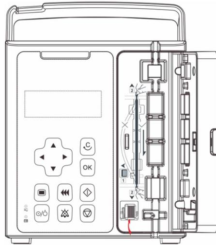
2. Pull the free flow clamp button upward left, and open the free flow clamp.
