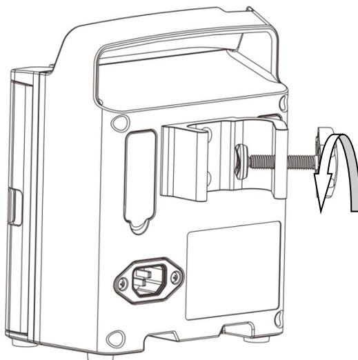
1. Turn counterclockwise to loosen the pole clamp until an IV stand can be inserted in.
