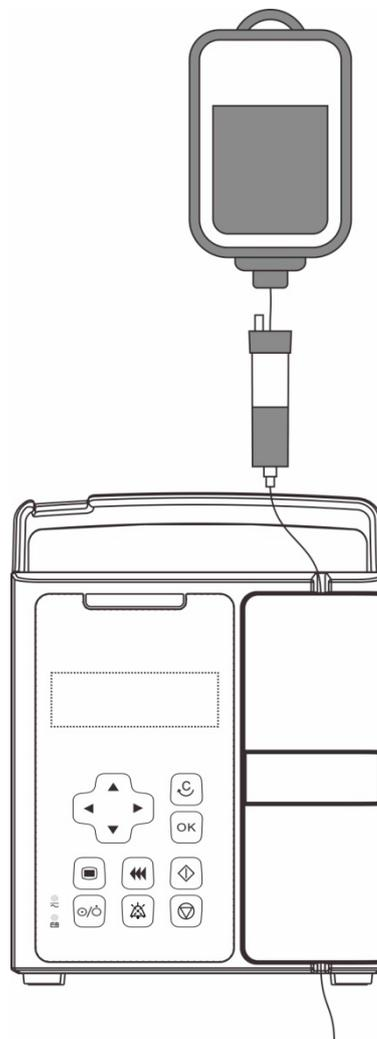
4. Close the door, the interface will enter **[Infusion set selection]** interface, indicating that the infusion set is loaded correctly; otherwise, it needs to be
