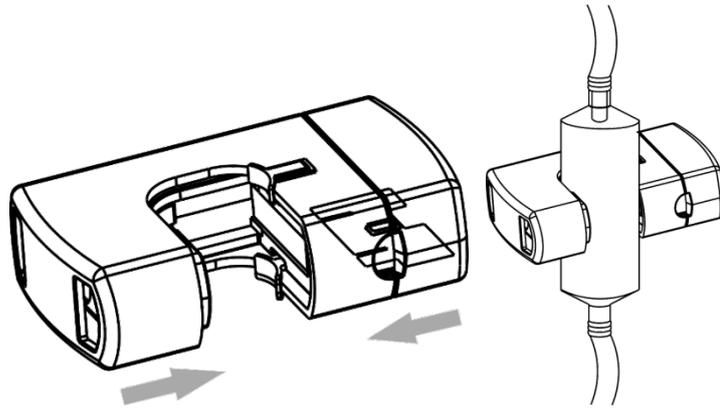
1. Firmly insert the signal line of drop sensor into the connecting port on the right side panel of the pump.
