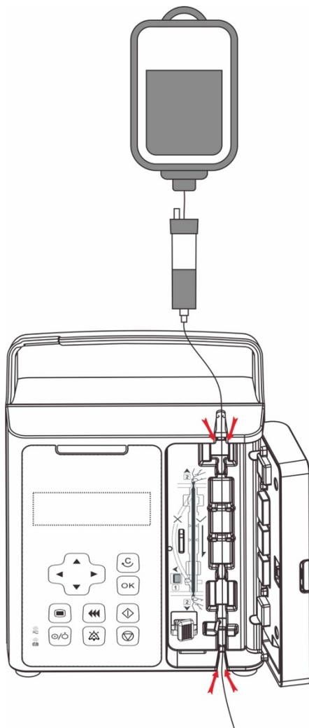
3. Load the set, confirm it is firmly loaded into the tube slot.
