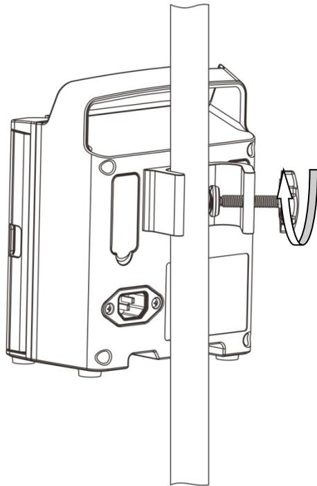
2. Tighten the pole clamp clockwise to firmly fix the device on the IV stand (round vertical bar with diameter size of 15-32mm).
